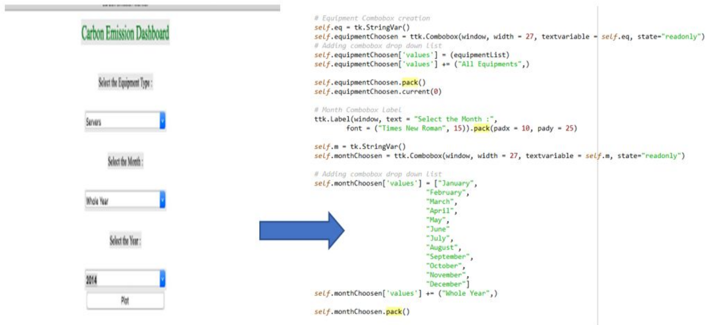
Figure 7 :part of the program code for the combo boxes
